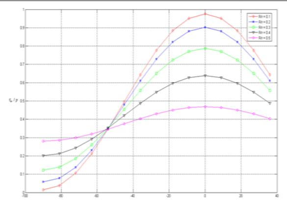
Fig. 2 Distribution of the Stress Component  $\tau_{\rm rr}$  Round the Edge of a Circular Hole
